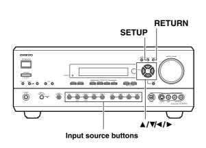
This menu allows you to make the various settings concerning the signals input from the various input sources that you use with the TX-SR701/701E/601/601E. The settings made in this menu are valid for the input source that is currently selected with the input source buttons at the front panel and, therefore, these settings are made separately for each input source.
